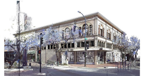
Figure 1: 3D point cloud overlaying the 3D BIM model.
