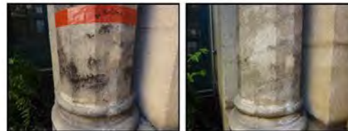
Test Panel 4, Triton X-114, before and after cleaning. (ARG/CS, 2011)
