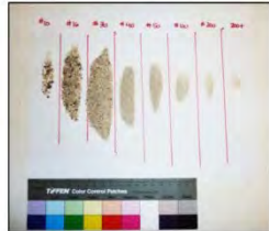
Particle-size distribution of Encina Commons plaster aggregate. (ARG/CS, 2011)
