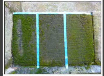
Area II, after pre-wetting and before application of biocides. (ARG, 2012)
