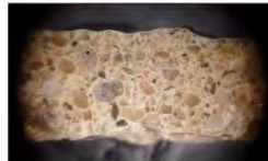
Photograph of Encina Commons plaster sample cross-section. (ARG/CS, 2011)
